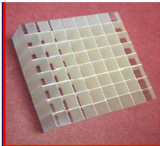
Standard Detector 6.4 mm x 6.4 mm 64 crystals/block
